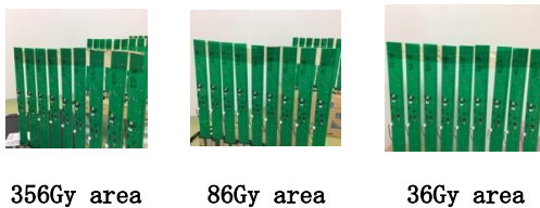
Fig. 1, Substrate with different irradiation amount
